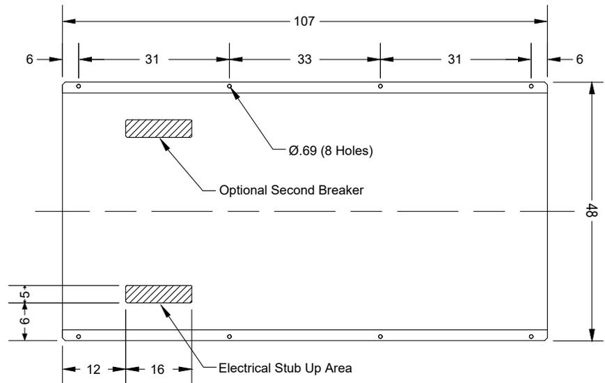
*Note: The above drawings are provided for reference only and should not be used for planning installation. Contact your local distributor for more information.*
